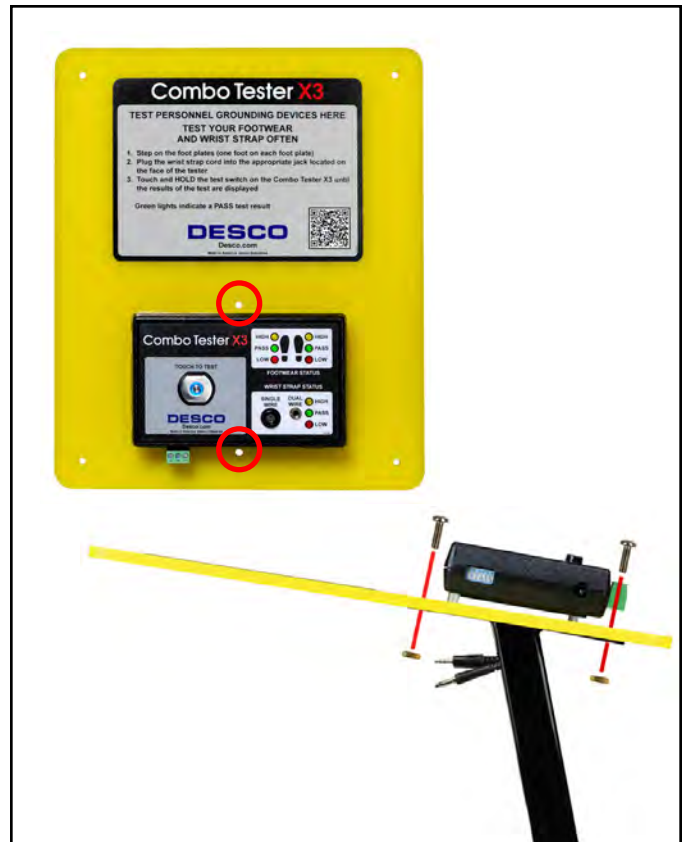
Figure 7. Securing the Combo Tester X3 to the pedestal
